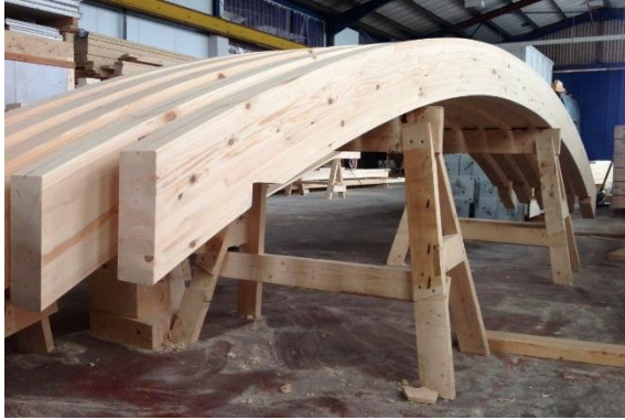
Fig 1.2. Curbed Glulam beams ;source//:novocom.top
