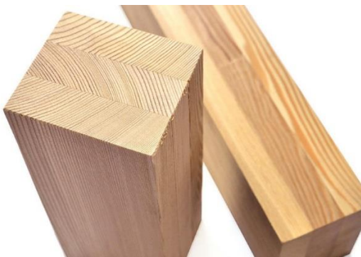
Fig 1.1: An Example of Glued Laminated Timber
